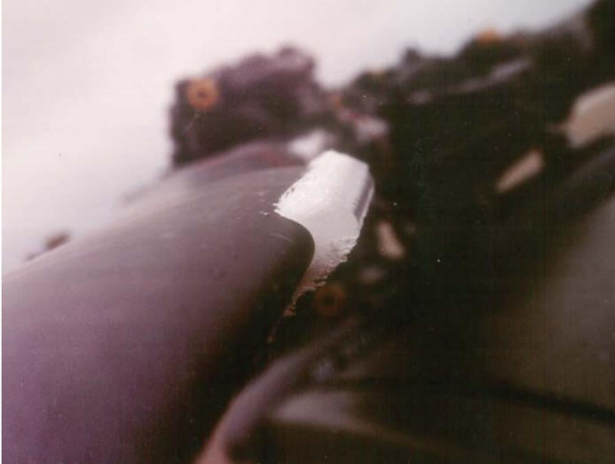
Approx 2 inches of ice on a leading edge. Not much in fixed wing terms but remember the size of the helicopter's 'wing' (rotor blade).
