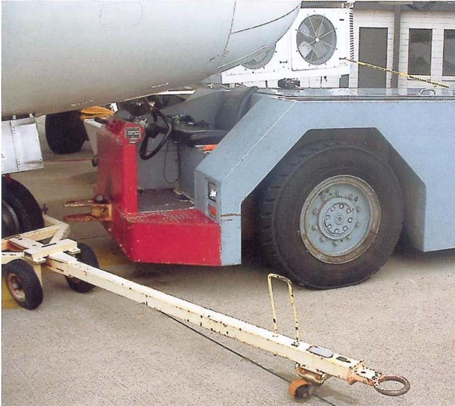
*A ramp worker lost his life while preparing to push back this DC-9 in December 2003. The tractor's operator left his seat to set the tow bar for attachment to the tug. On return, his foot accidentally hit the accelerator and the tug jumped forward and struck the aircraft radome, fatally pinning the driver. The driver had failed to set the parking brake before leaving the tug.*
