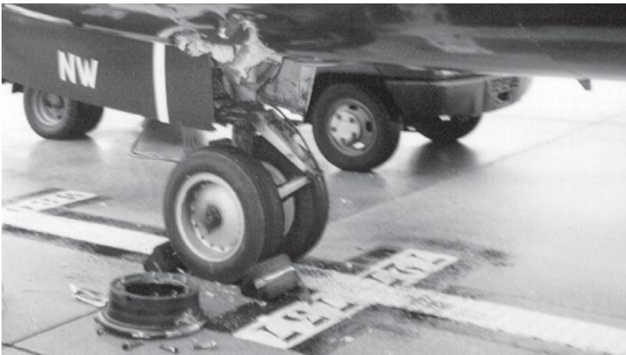
*Split hub lying below the hole in the fuselage*
