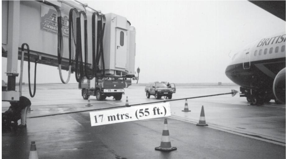
*Position of air jetty to aircraft when jetty wheel failed*
