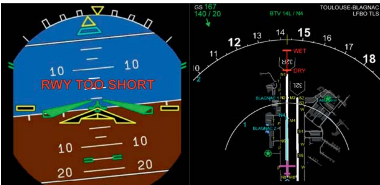
Figure 4: Illustration of PFD and ND (ARC mode in Airport Navigation range) in case of “Dry” ROW alert
