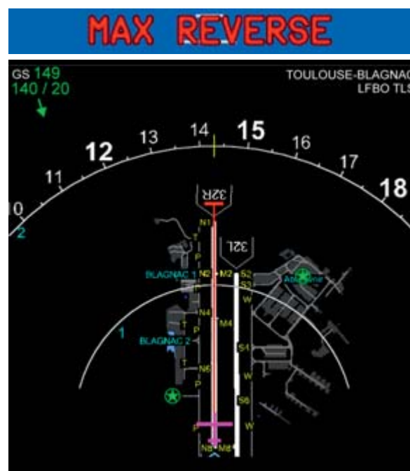
Figure 6: Illustration of PFD and ND (ARC mode in Airport Navigation range) in case of ROP alert
