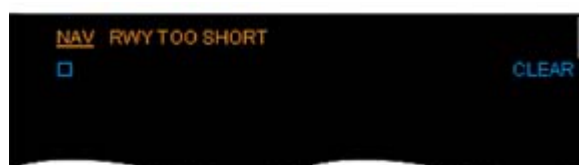
Figure 8: ECAM alarm when the Lift-off run check detects a risk of overrun at take-off (take-off power condition is false)
