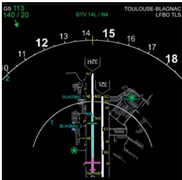
Figure 5: Illustration of ND (ARC mode in Airport Navigation range) in normal condition
