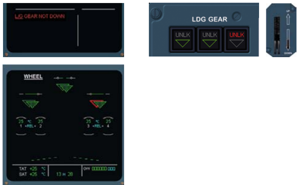
Figure 6 Illustration of spurious “ L/G GEAR NOT DOWN” indication
