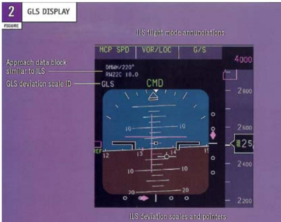
The new navigation options work together or separately to enable pilots to fly safe, stable, and precise three-dimensional paths that smoothly intercept a variety of final approach legs.
