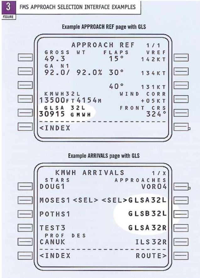
character approach identifier to ensure consistency between the selected channel and the approach procedure chosen by the pilot. The approach identifier is read from the FAS data block and displayed to the pilot on the PFD to provide positive confirmation that the desired approach has indeed been selected.
