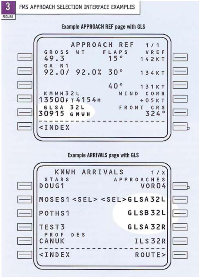
using a designated VHF navigation frequency. As with the ILS certain GLS identification data are available on other FMS pages such as the APPROACH REF page, which shows the runway identifier, GLS channel, and associated approach identifier (fig. 3).
